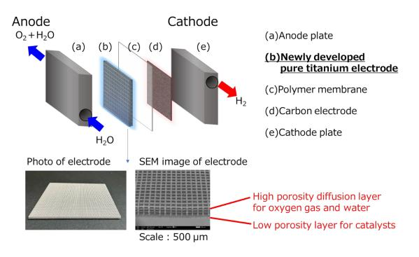
Schematic diagram of PEM water electrolysis
